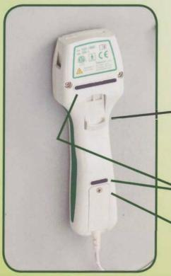
Handpiece Latch. When the latch is pushed in the "down" position, the latch retracts the contact pins inside the Handpiece to allow insertion of the sensor tab. When Pushed "up" the sensor is fully inserted and locked in place.
